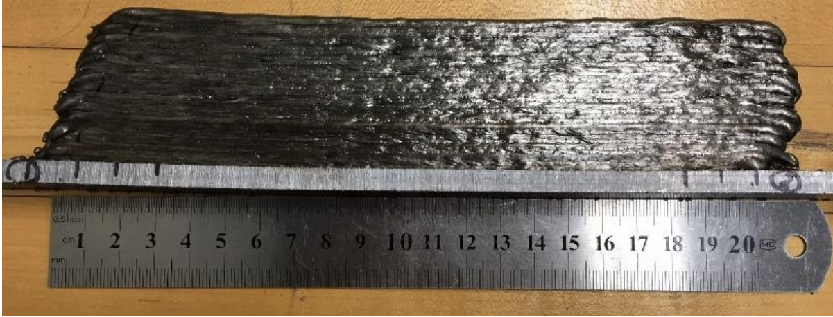
Figure 7. The final AM part in scale (Done at Clarkson University)
