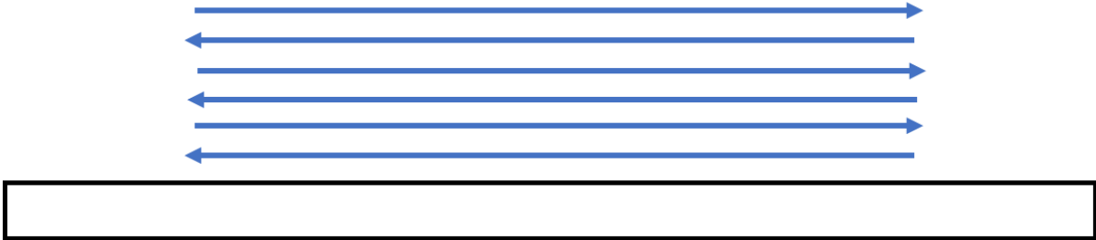
Figure 5. Illustration of welding direction for WAAM wall
