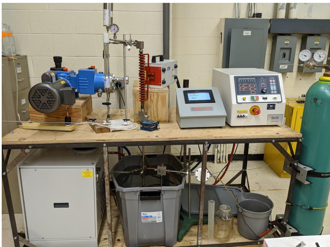
Figure 4. Mobile algae processing pilot unit
