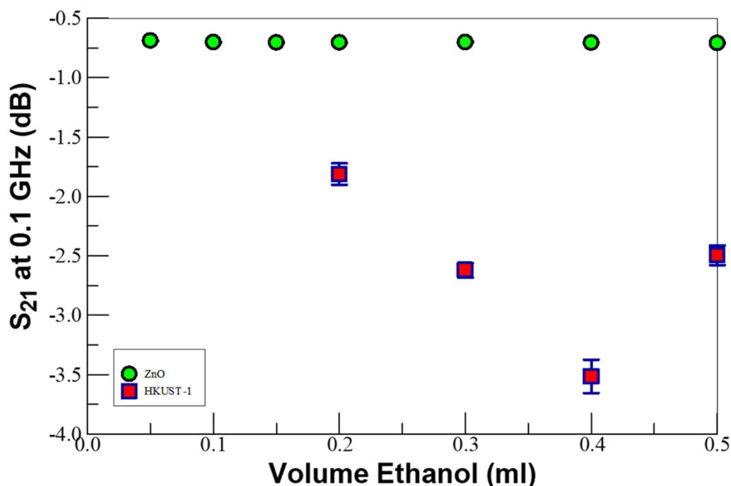
**Figure 4.** Comparison of the microwave insertion loss ( $S_{21}$ ) dependence on ethanol concentration on ZnO versus TCNQ-doped-HKUST-1 MOF on Si in gaseous ethanol environments, monitored at 0.1 GHz. Note the error bars represent the standard deviation of at least 3 replicate measurements.
