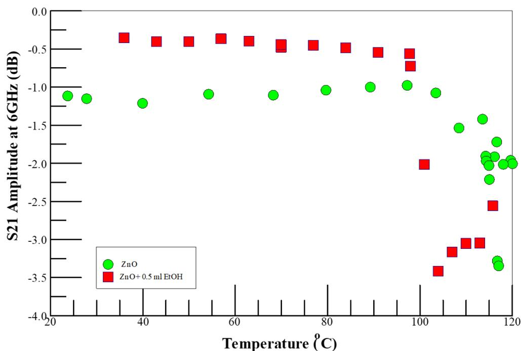
**Figure 1.** Temperature dependence of microwave insertion loss (S21 amplitude) of ZnO on Si substrate in nitrogen-rich air and gaseous ethanol environments, monitored at 6 GHz. Note that the symbol sizes are much larger than the error bars.
