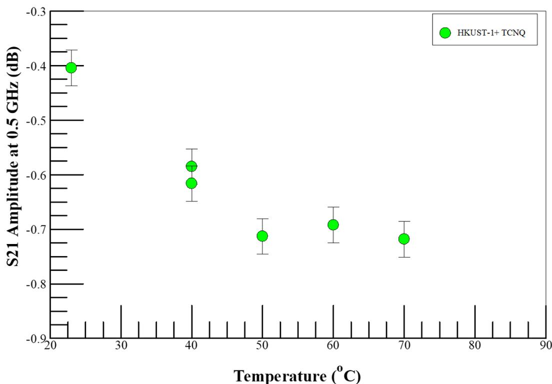
**Figure 2.** Temperature dependence of microwave insertion loss ( $S_{21}$  amplitude) in TCNQ-loaded HKUST-1 MOF on a Si sample in  $\text{N}_2$ -rich air. The error bars represent the standard deviation of three or more measurements on the same sample.
