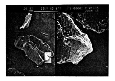
hammered edges (Figure 13c). Many grains of this type exhibit a shingled appearance (Figure 13b) which is probably due to crystalization or slippage along weaker crystal plains. Each layer or shingle is delicately connected to its adjacent shingle.
