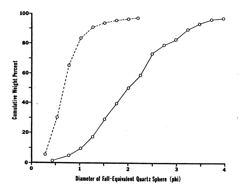
Figure 12. Comparison of size distributions based on sieve analysis to those generated by RSA analysis for the Panambisito gravel sample. Upper graph shows sieve sizes, lower graph shows settling sizes. Dashed lines = gold, solid lines = black sands.
