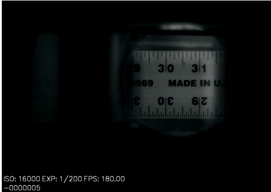
Figure 22: Calibration image for pixel to meter conversion.
