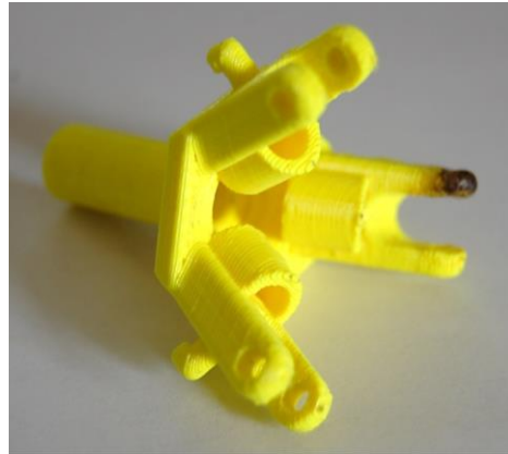
Figure 16: 3D printed Mark 1 grabber base for MSBS testing.
