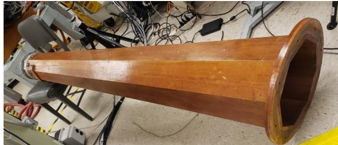
Figure 6: Removeable section of diffuser.
