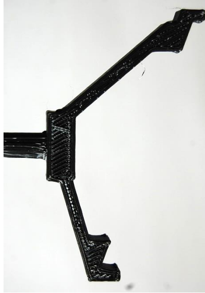
Figure 20: 20-degree edge holder for Stardust MSBS testing.
