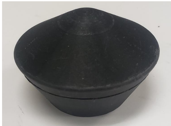
Figure 21: 3D printed Stardust model. [Heatshield (front) side up]
