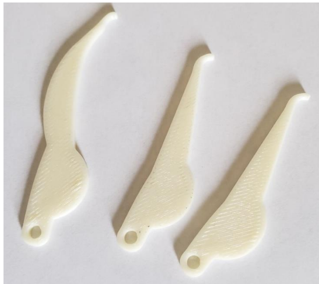
Figure 72: Mark 2 3D printed long gripper and short grippers for MSBS testing.
