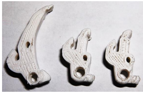
Figure 12: Mark 1 3D printed long gripper and short grippers for MSBS testing.
