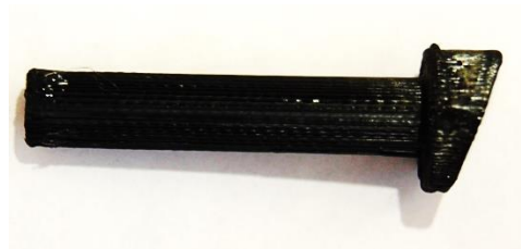
Figure 19: 20-degree standard sting for Stardust MSBS testing.
