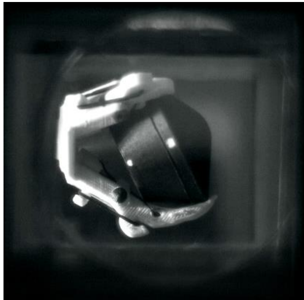
Figure 29: Mark 1 grabber holding Stardust capsule for free to oscillate testing.
