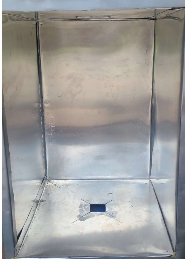
Figure 3. The convective heating chamber where high temperature testing was performed.
