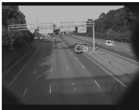
Figure 4. The output of the feature tracking algorithm. (a) The output from the feature tracking algorithm with a bounding box around the feature and the object number identified
