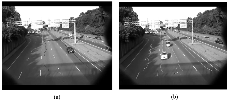
Figure 5. One example output of the trajectory clustering algorithm. (a) Early outputs in training with dark lines indicating clusters which have only a few trajectories. (b) Output after several hundred more frames with the light colored lines indicating clusters with multiple trajectories.
