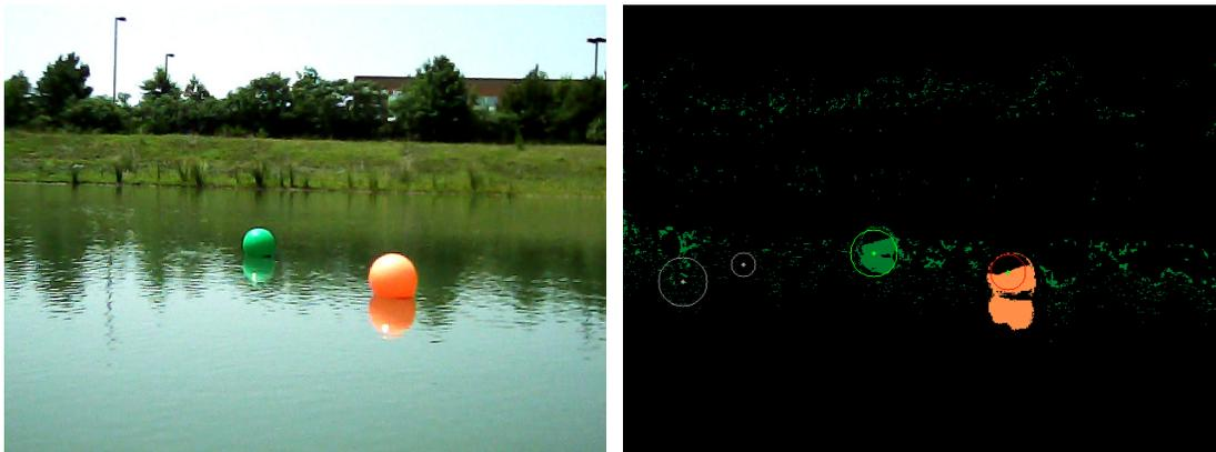
**Figure 4. Maritime Test. a) Field Image. b) Buoy Prediction**
