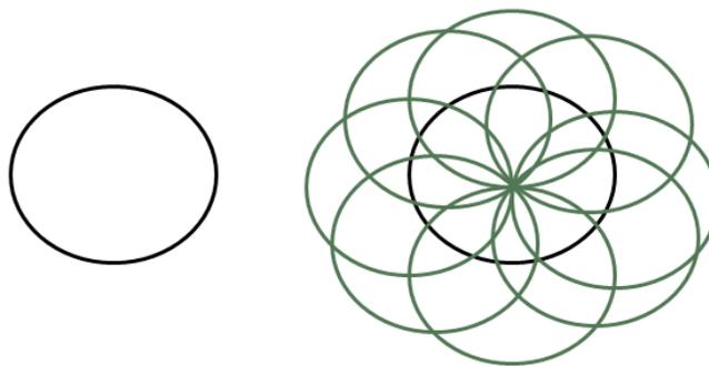
**Figure 2. Circular Hough Transform. a) Original Circle. b) Secondary Circles**
