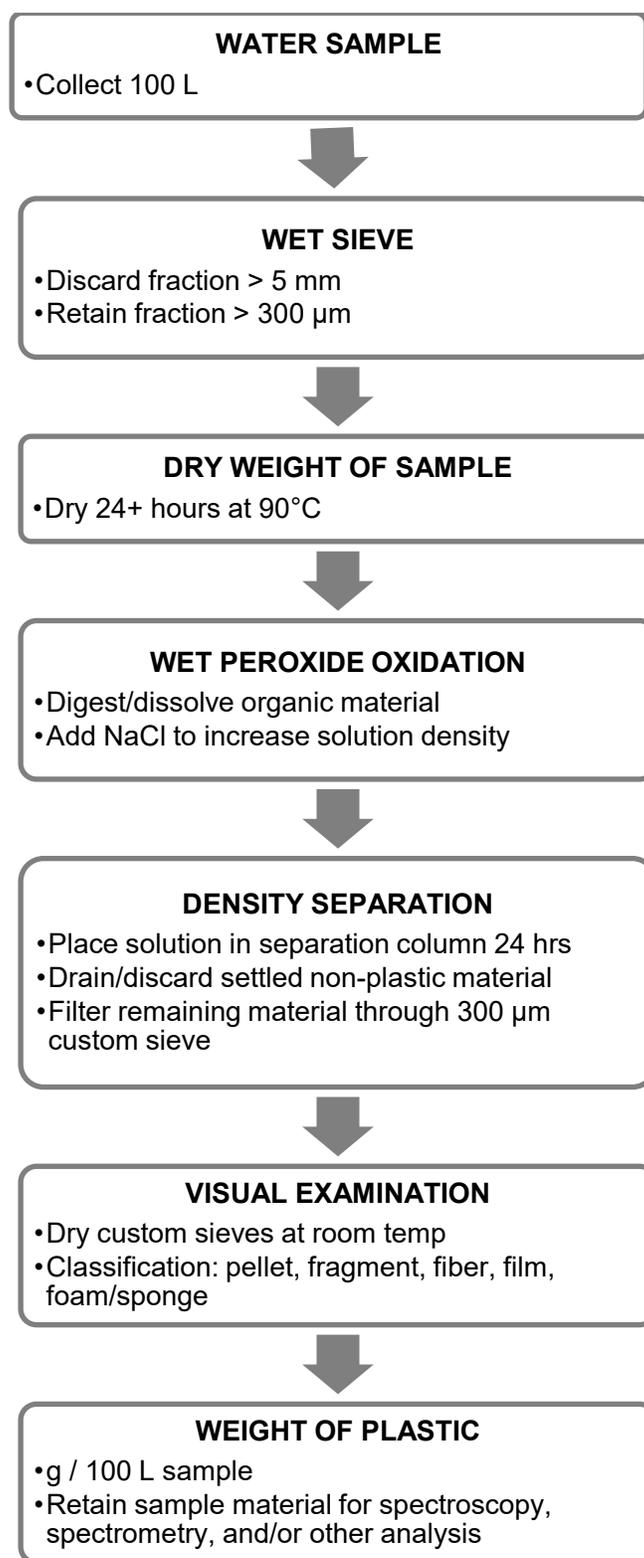
**Figure 3:** Flow chart of sample collection/analysis procedure
