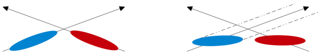
FIG. 1. Bunches colliding with a crossing angle without crab crossing (left); with the crab crossing (right).
