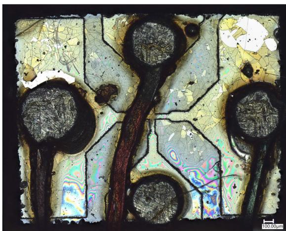
FIG. 1. Optical microscopy image of the active area of the Hall probe sensor HHP-VFS.
