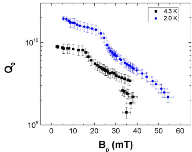
Figure 8:  $Q_0(B_p)$  measured at 4.3 K and 2.0 K after depositing a ~5 mm thick Cu layer on the cavity outer surface<sup>1</sup>. The cavity was limited by quench at 2.0 K.
