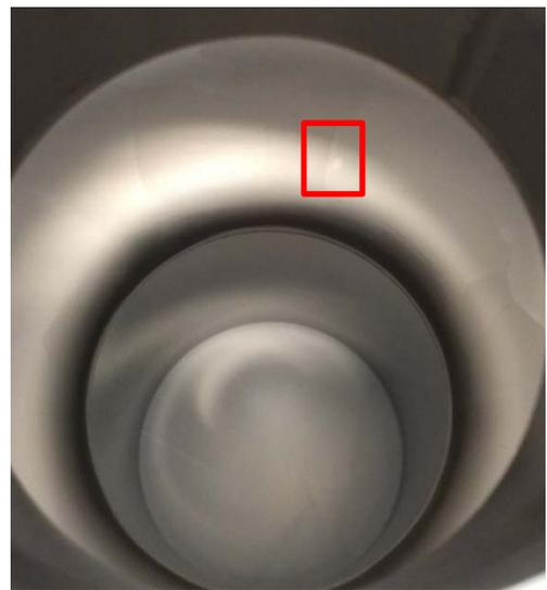
Figure 3: A picture of SC-IB interior after second Nb<sub>3</sub>Sn coating. Note the shiny spot marked by red rectangle.
