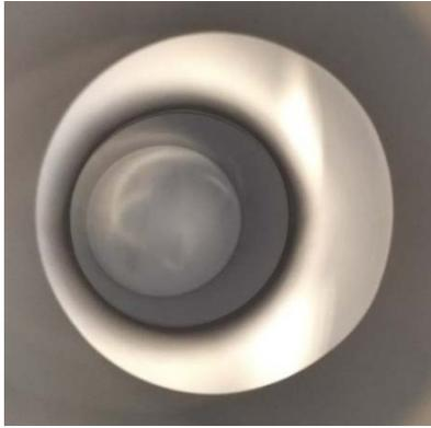
Figure 1: A picture of SC-IB interior after Nb<sub>3</sub>Sn coating.
