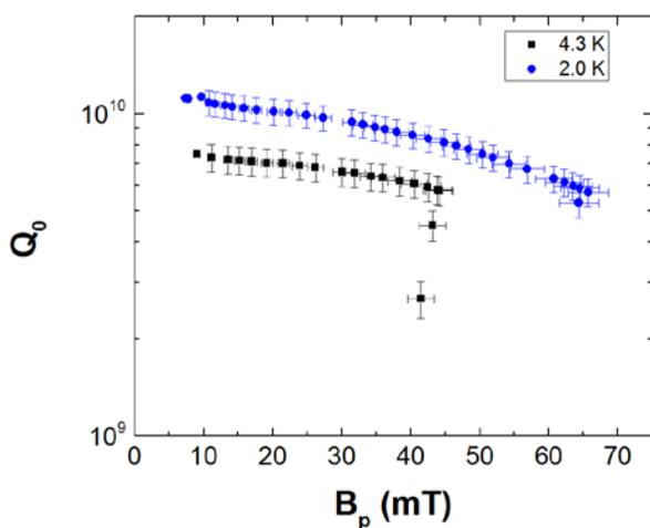
Figure 2:  $Q_0(B_p)$  measured at 4.3 K and 2.0 K after the first Nb<sub>3</sub>Sn coating<sup>1</sup>. The cavity was limited by anomalous heating at 4.3 K and by quench at 2.0 K.
