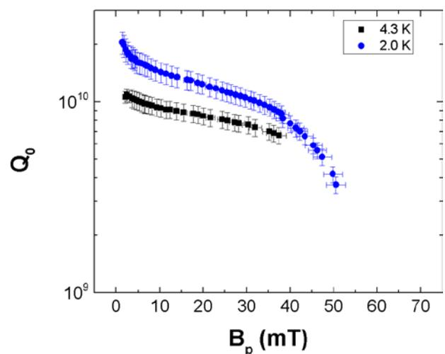
Figure 4:  $Q_0(B_p)$  measured at 4.3 K and 2.0 K after the second Nb<sub>3</sub>Sn coating<sup>1</sup>. The cavity was limited by quench at 2.0 K.
