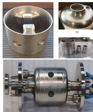
Figure 8: Machined sub-assemblies (top) and fabricated (bottom) 650 MHz rf-separator.
