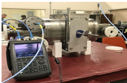
Figure 8: Setup for measuring tuner sensitivity for rf-dipole cavity.
