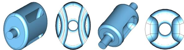
Figure 4: 400 MHz (left) and 750 MHz (right) crabbing cavities.
