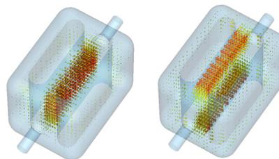
Figure 2: Electric field (left) and magnetic field (right) profiles for the rectangular shaped parallel-bar cavity.
