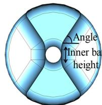
Figure 2: Optimized design parameters of the bars in the parallel-bar geometry.
