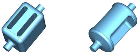
Figure 1: Rectangular shaped (left) and cylindrical shaped parallel-bar geometries.
