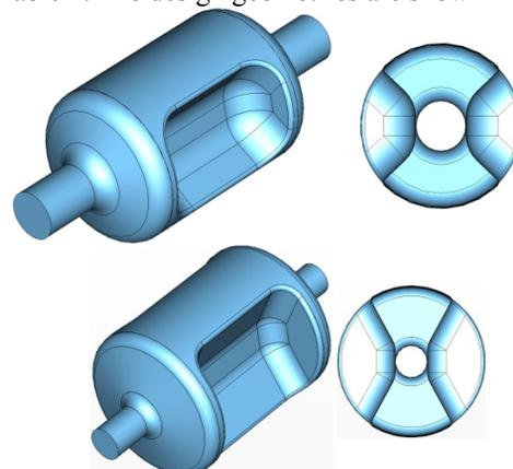
Figure 7: 750 MHz crabbing cavity (top) and 365.625 MHz deflecting cavity (bottom).
