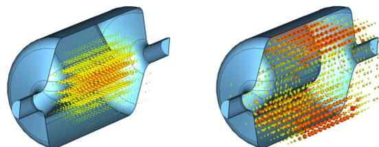
Figure 3: Electric field profile (left) and magnetic field profile (right) of the parallel-bar cavity.
