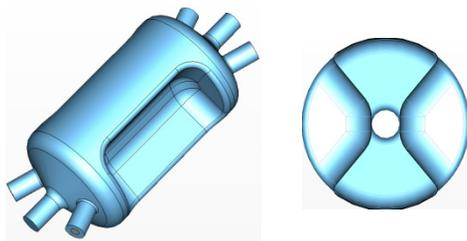
Figure 5: 499 MHz deflecting cavity (left) and the cross section (right).
