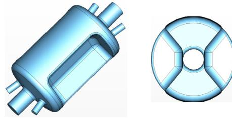
Figure 6: 400 MHz crabbing cavity (left) and the cross section (right).
