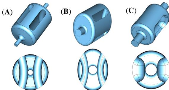
Figure 1: Parallel-bar cavity designs. (A) 499 MHz cylindrical shaped design with curved bars, (B) 400 MHz elliptical shaped design with curved bars and (C) 750 MHz cylindrical shaped design with bars merged on to the walls (top) and vertical cross section of each design (bottom).
