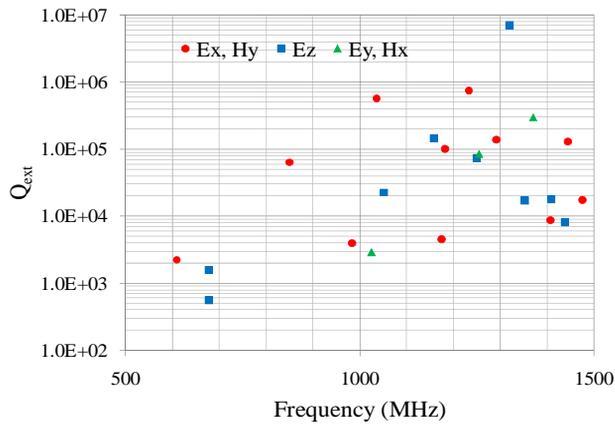
Figure 6: Required  $Q_{ext}$  for HOMs to achieve the specified damping.
