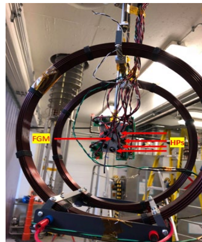
Figure 1: Hall probes calibration setup.
