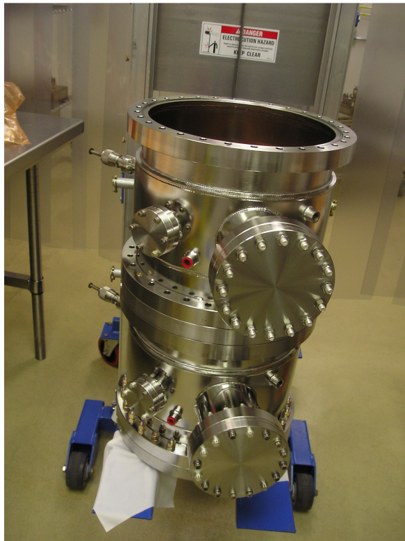
Figure 2: Clean room assembly of separator cavity.
