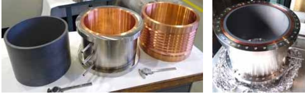
Figure 19. Dielectric beam line absorber with shrink-fit cooling jacket.
