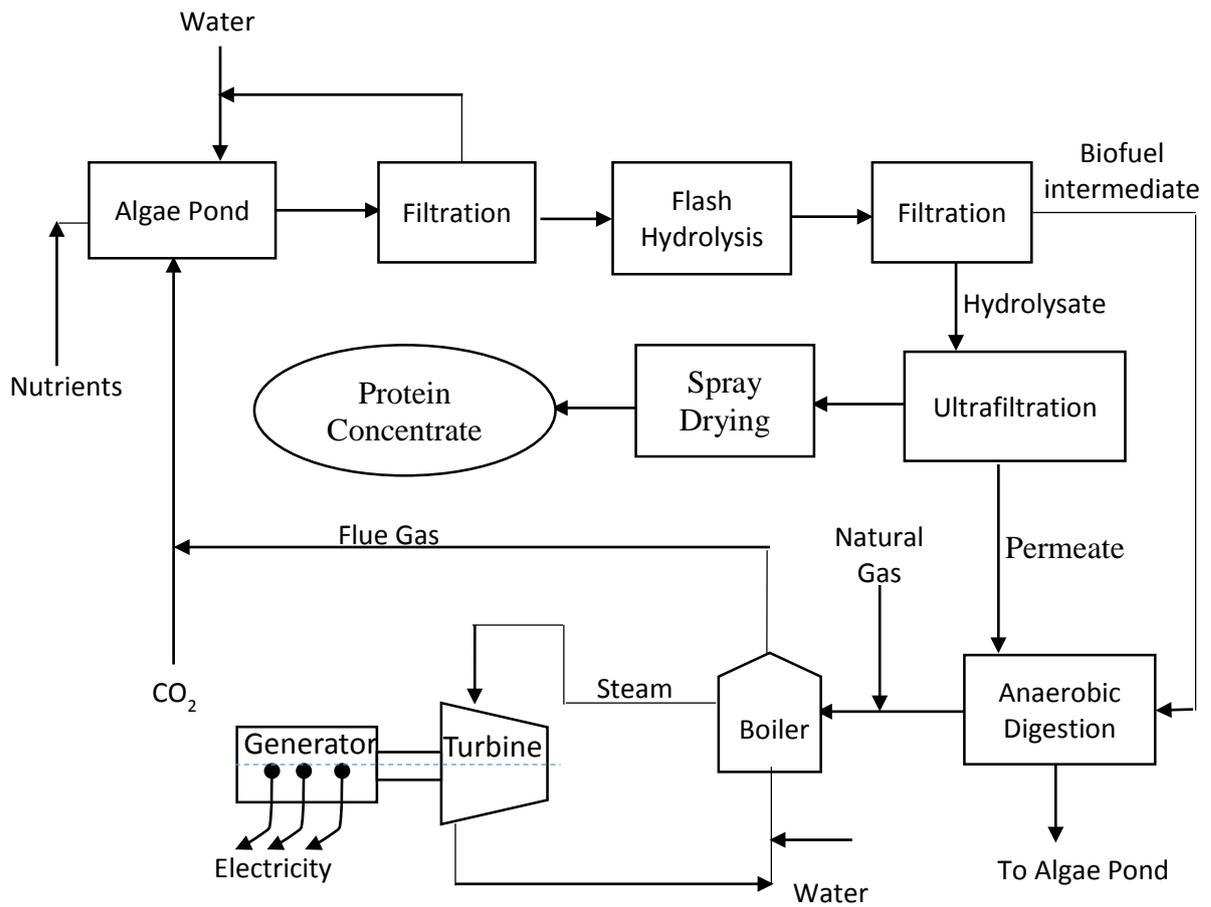
Figure 2. Simplified Process flowsheet for protein concentrate production.
