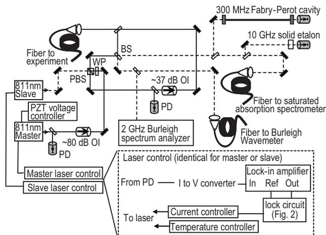
FIG. 1. Schematic of experimental setup. PBS: polarizing beamsplitter cube; BS: beamsplitter; WP: waveplate; OI: optical isolator; PD: photodiode; dashed optical path indicates master and slave laser beam overlap.
