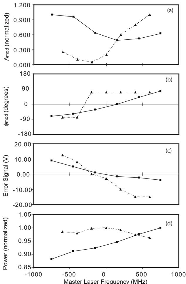
FIG. 4. For master laser (squares) and slave laser (triangles): (a) normalized  $A_{mod}$  vs laser frequency, (b)  $\phi_{mod}$  vs laser frequency, (c) output of the lock-in amplifier (used as the error signal) vs laser frequency, and (d) normalized total laser power vs laser frequency.
