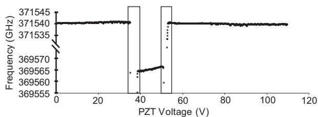
FIG. 3. Output frequency of slave laser without electronic feedback vs master laser PZT voltage (corresponding to master laser frequency). Boxed region indicates multimode behavior.
