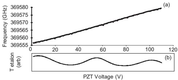
FIG. 5. (a) Output frequency of slave laser with electronic feedback vs master laser PZT voltage (b) Transmission of slave laser light through a 10 GHz solid etalon vs master laser PZT voltage.
