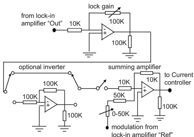
FIG. 2. Amplifier circuit with gain and polarity control for providing combined modulation and error signal to the diode laser current controller. All operational amplifiers are 1/4 TL074.
