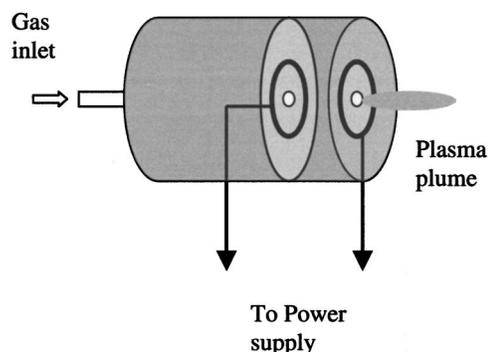
FIG. 1. Schematic of the plasma pencil.
