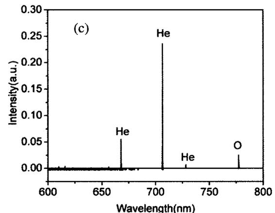
FIG. 4. Emission spectra: (a) 280–400 nm range showing OH,  $N_2$ , and  $N_2^+$  emission lines; (b) 400–600 nm showing  $N_2$ ,  $N_2^+$  and He lines; (c) 600–800 nm range showing He and O lines.
