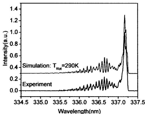
FIG. 3. Experimental and simulated emission spectra of  $N_2$  second positive system. The curves are shifted intentionally for better comparison.
