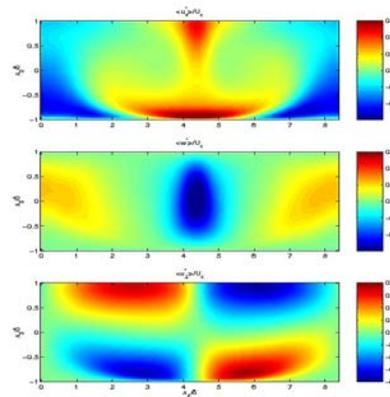
**Figure 2.** Contours of the vertical and cross-stream distribution of the mean turbulent velocity fluctuations. The panels show, from top to bottom, the streamwise, the vertical and the cross-stream velocity components. The depth (0 to  $-H$ ) has been scaled by the half depth and mapped into  $-1$  to  $1$ . The width is also scaled by the half depth.
