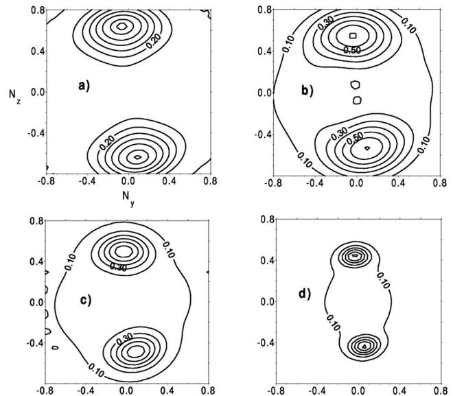
FIG. 7. Contour maps of absorbed power in MAST at various frequencies for optimal oblique incidence of linearly polarized wave for H-mode operation (see Fig. 3). (a)  $f = 18$  GHz,  $\alpha = 41^\circ$ , (b)  $f = 30$  GHz,  $\alpha = 35^\circ$ , (c)  $f = 40$  GHz,  $\alpha = 31^\circ$ , and (d)  $f = 50$  GHz,  $\alpha = 26^\circ$ .
