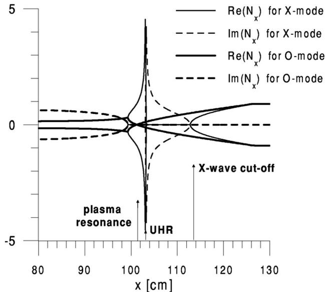
FIG. 4. WKB solution of the cold dispersion equation for optimal launch into a simple parabolic MAST density profile, Fig. 1,  $N_y = 0.11$ ,  $N_z = 0.42$  ( $\alpha = 25^\circ$ ),  $f = 60$  GHz and weak collisions:  $\nu/\omega = 10^{-4}$ .
