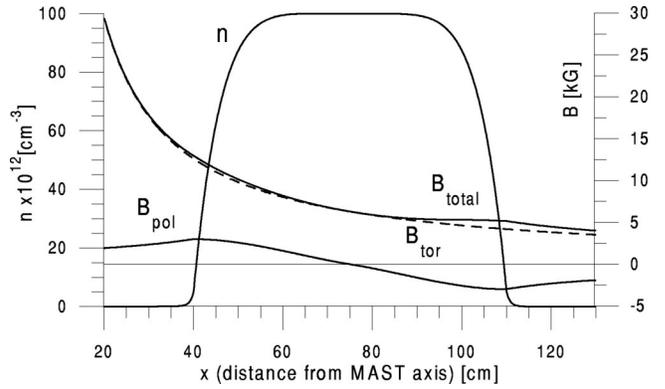
FIG. 3. The narrow flat density and magnetic field profiles corresponding to the formation of a H-mode transport barrier in MAST.
