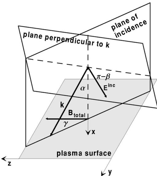
FIG. 2. The geometry of a linearly polarized electromagnetic wave incident on a plasma.
