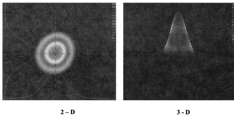
FIG. 5. 2D and 3D beam profile.
