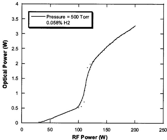
FIG. 4. Total optical power dependence on the input rf power at pressure of 500 Torr.
