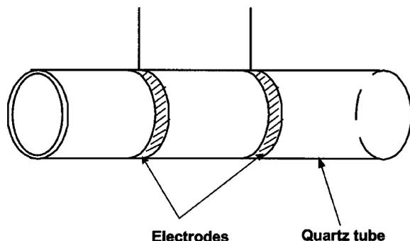
FIG. 1. Cylindrical DBD configuration with ring electrodes.
