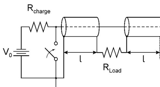
Pulse generators based on the Blumlein concept are line-type pulsers (Figure 1). For short pulses (less than 100 ns) the pulse forming lines consist of two strip lines or two coaxial cables of equal length,  $l$ , with the total length determined by the desired pulse duration,  $\tau$ :
